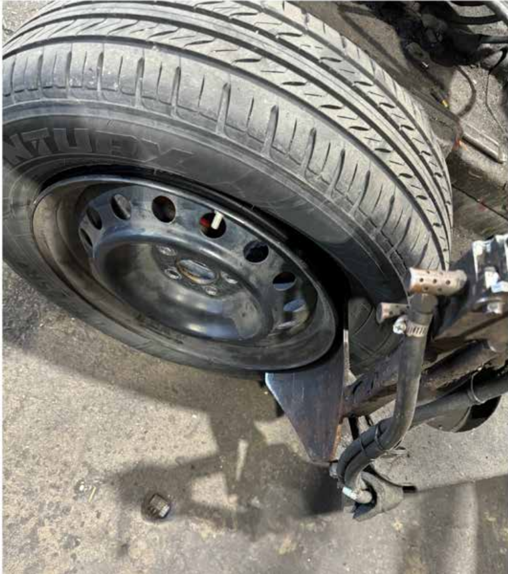
Picture of breaking the front bead from the rim flange
