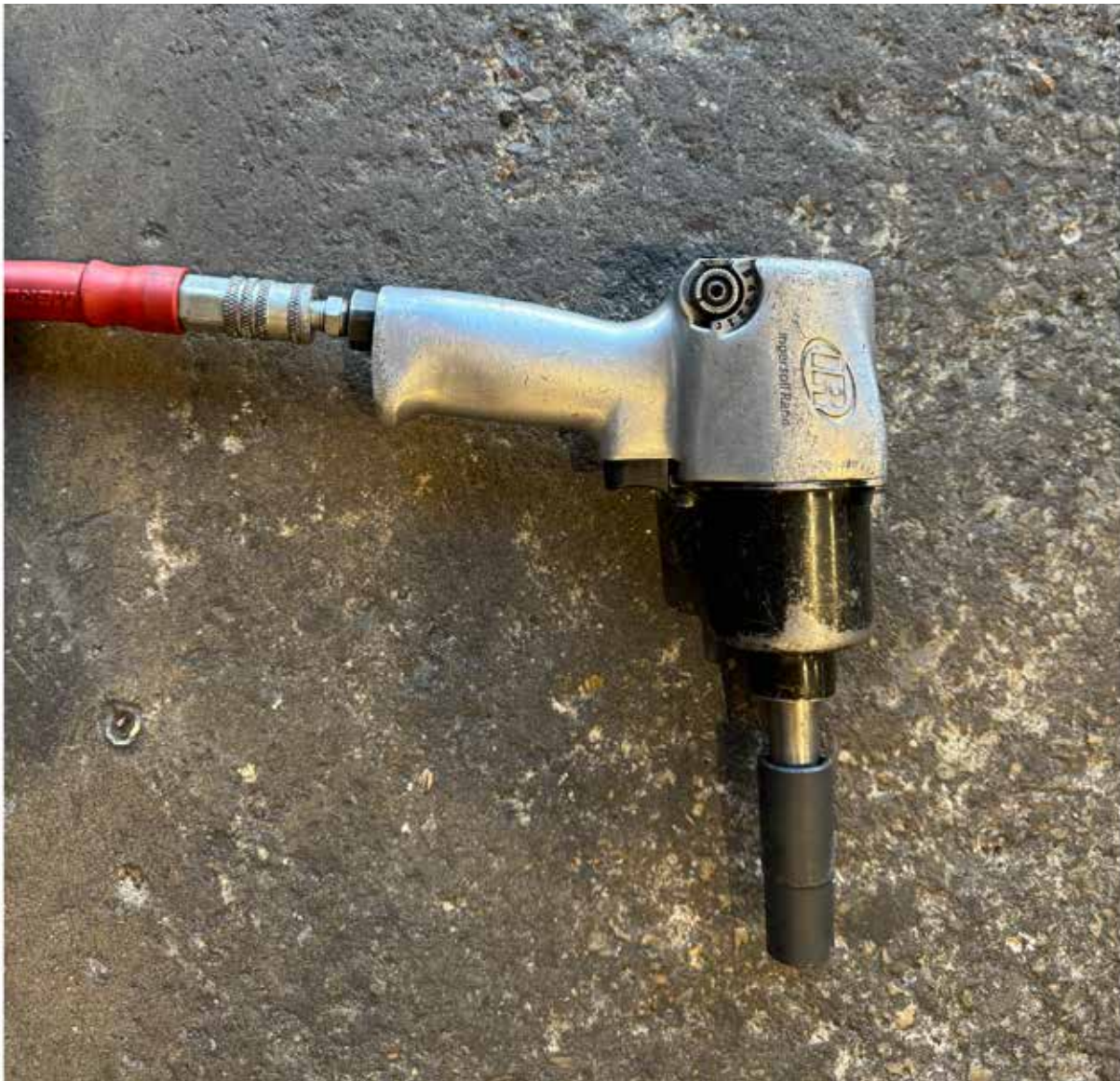
Picture 11. PNEUMATIC 1/2" IMPACT WRENCH WITH FLIP SOCKET AND AIR LINE ATTACHED
