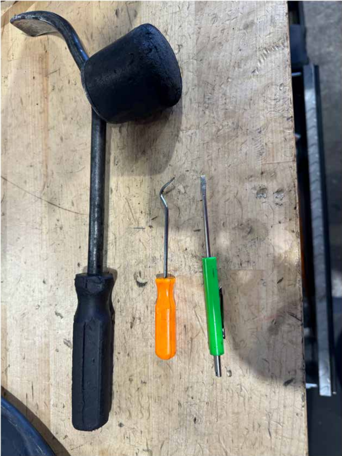
Picture 7. Hubcap Tools to remove wheel cover
