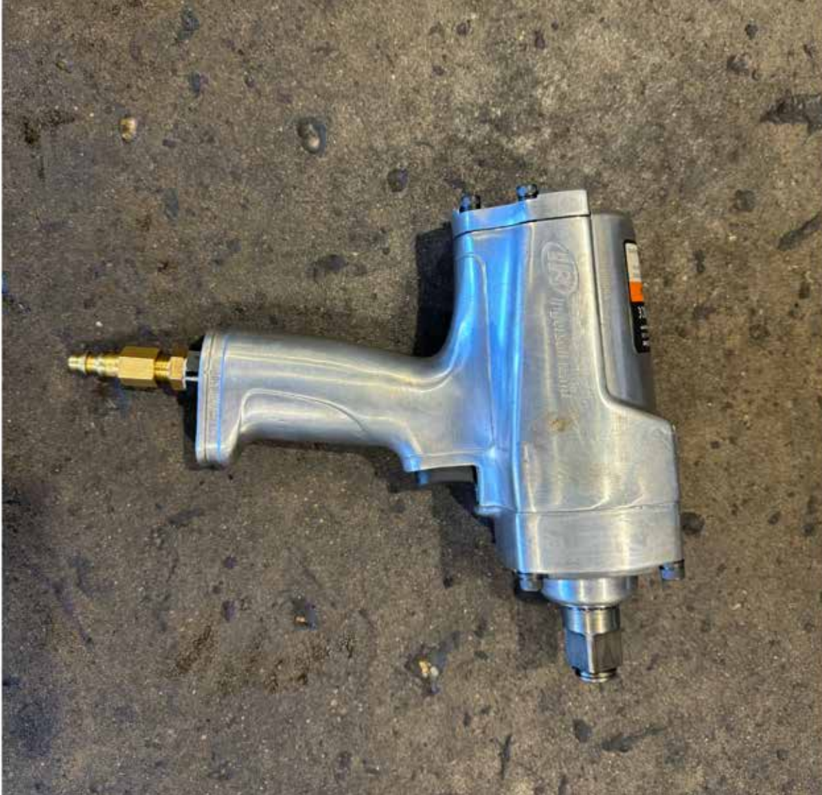
Picture 13. 3/4" pneumatic impact wrench for larger trucks
